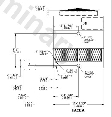
**SHIPPING** OPERATING HEAVIEST SECTION 6690 lbs+ [3035] kg+ 11650 lbs+ [5285] kg+ WEIGHT WEIGHT WEIGHT
