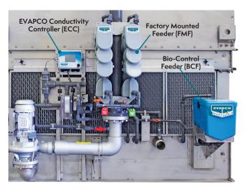
EVAPCO's **Smart Shield**® system utilizes proven solid chemistry delivered via our revolutionary feed system. With patented Controlled Release tablets, a scale and corrosion inhibitor is fed whenever your spray water pump is energized. Thus keeping your system protected anytime the spray water pump is operating.
