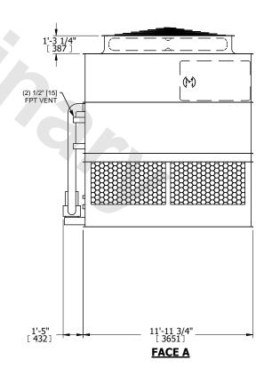
DRAWN BY: SLR NO. OF SHIPPING SECTIONS **SHIPPING** OPERATING HEAVIEST SECTION 12520 lbs+ [5680] kg+ 20030 lbs+ [9090] kg+ 9970 lbs+ [4525] kg+ WEIGHT WEIGHT WEIGHT
