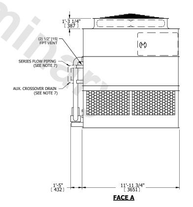
DRAWN BY: NO. OF SHIPPING SECTIONS **SHIPPING OPERATING** HEAVIEST SECTION 12390 lbs+ [5625] kg+ 19900 lbs+ [9030] kg+ 9840 lbs+ [4465] kg+ WEIGHT WEIGHT WEIGHT
