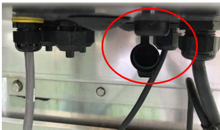
Figure 3. USB Port with Protective Cover Open
