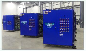
Purity Rack Highlighting Microprocessor Control Panels
