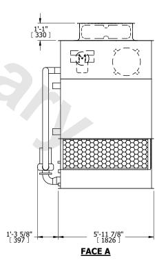
DRAWN BY: NO. OF SHIPPING SECTIONS **SHIPPING OPERATING** HEAVIEST SECTION 3570 lbs+ [1620] kg+ 4810 lbs+ [2185] kg+ 3060 lbs+ [1390] kg+ WEIGHT WEIGHT WEIGHT
