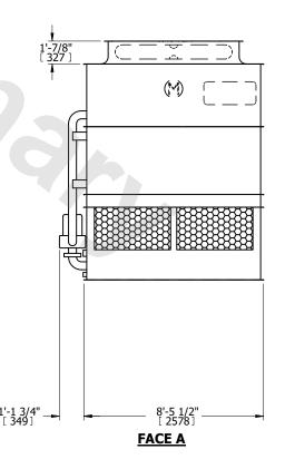
DRAWN BY: SLR NO. OF SHIPPING SECTIONS **SHIPPING** OPERATING HEAVIEST SECTION 7780 lbs+ [3530] kg+ 6480 lbs+ [2940] kg+ 10380 lbs+ [4710] kg+ WEIGHT WEIGHT WEIGHT
