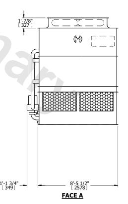
**SHIPPING** OPERATING HEAVIEST SECTION 6490 lbs+ [2945] kg+ 7790 lbs+ [3535] kg+ 10390 lbs+ [4715] kg+ WEIGHT WEIGHT WEIGHT
