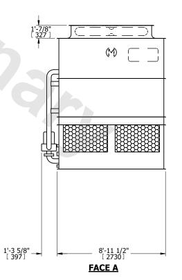
NO. OF SHIPPING SECTIONS **SHIPPING** OPERATING HEAVIEST SECTION 7750 lbs+ [3520] kg+ 9190 lbs+ [4170] kg+ 12210 lbs+ [5540] kg+ WEIGHT WEIGHT WEIGHT
