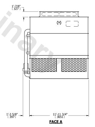
DRAWN BY: SLR NO. OF SHIPPING SECTIONS **SHIPPING** OPERATING HEAVIEST SECTION 14960 lbs+ [6790] kg+ 13160 lbs+ [5970] kg+ 19380 lbs+ [8795] kg+ WEIGHT WEIGHT WEIGHT
