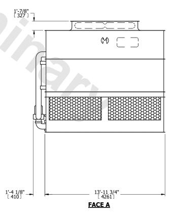
DRAWN BY: SLR NO. OF SHIPPING SECTIONS **SHIPPING** OPERATING HEAVIEST SECTION 13110 lbs+ [5950] kg+ 15120 lbs+ [6860] kg+ 20110 lbs+ [9125] kg+ WEIGHT WEIGHT WEIGHT
