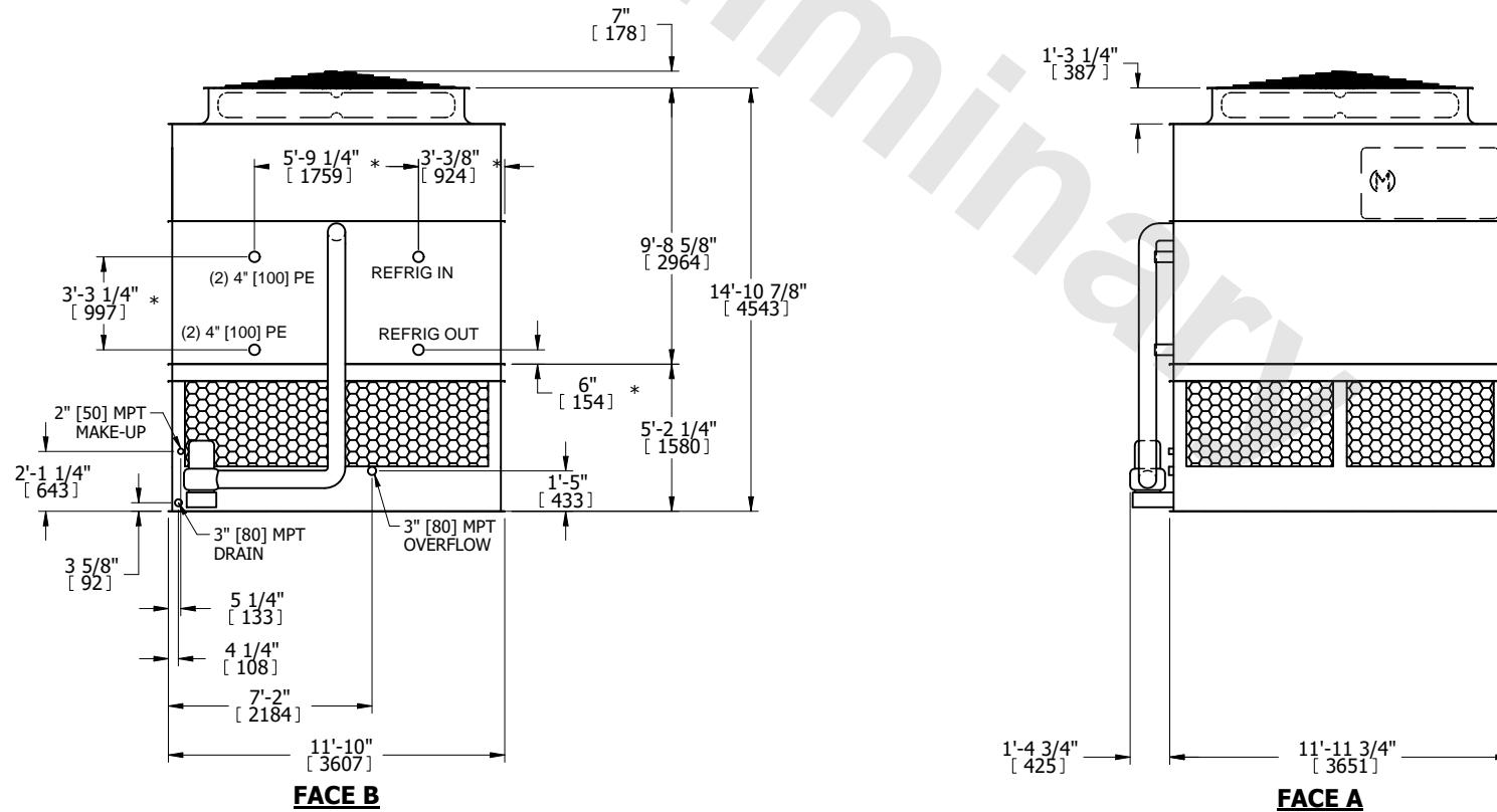
SHIPPING WEIGHT 18830 lbs+ [8545] kg+ OPERATING WEIGHT 25810 lbs+ [11710] kg+ HEAVIEST SECTION WEIGHT 16120 lbs+ [7315] kg+ NO. OF SHIPPING SECTIONS 2 DRAWN BY: SLR
