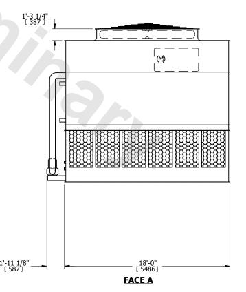
SHIPPING WEIGHT 30630 lbs+ [13895] kg+ OPERATING WEIGHT 41430 lbs+ [18795] kg+ HEAVIEST SECTION WEIGHT 26710 lbs+ [12120] kg+ NO. OF SHIPPING SECTIONS 2 DRAWN BY: SLR
