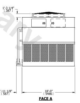
SHIPPING WEIGHT 54040 lbs+ [24515] kg+ OPERATING WEIGHT 75080 lbs+ [34060] kg+ HEAVIEST SECTION WEIGHT 23100 lbs+ [10480] kg+ NO. OF SHIPPING SECTIONS 4 DRAWN BY: SLR
