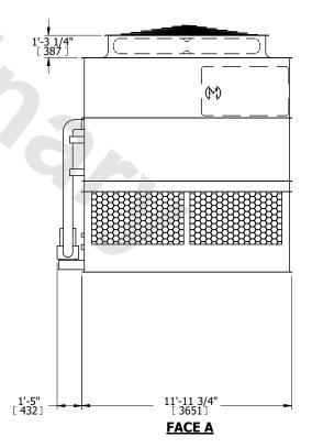
DRAWN BY: SLR NO. OF SHIPPING SECTIONS **SHIPPING** OPERATING HEAVIEST SECTION 12390 lbs+ [5625] kg+ 9840 lbs+ [4465] kg+ 18260 lbs+ [8285] kg+ WEIGHT WEIGHT WEIGHT
