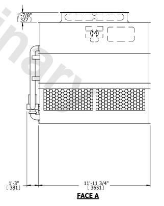
DRAWN BY: SLR NO. OF SHIPPING SECTIONS **SHIPPING** OPERATING HEAVIEST SECTION 11150 lbs+ [5060] kg+ 14800 lbs+ [6715] kg+ 9380 lbs+ [4255] kg+ WEIGHT WEIGHT WEIGHT
