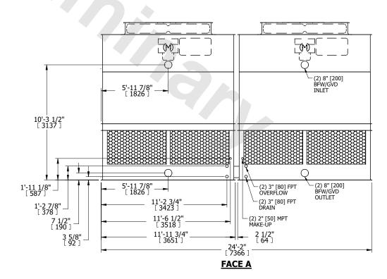
SHIPPING WEIGHT 12460 lbs+ [5655] kg+ OPERATING WEIGHT 20180 lbs+ [9155] kg+ HEAVIEST SECTION WEIGHT 4370 lbs+ [1985] kg+ NO. OF SHIPPING SECTIONS 4 DRAWN BY: JLG
