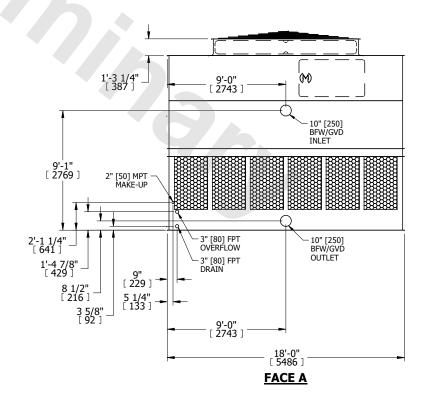
SHIPPING WEIGHT 10820 lbs+ [4910] kg+ OPERATING WEIGHT 20090 lbs+ [9115] kg+ HEAVIEST SECTION WEIGHT 6920 lbs+ [3140] kg+ NO. OF SHIPPING SECTIONS 2 DRAWN BY: KDS
