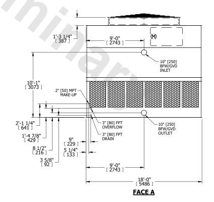
DRAWN BY: KDS NO. OF SHIPPING SECTIONS **SHIPPING OPERATING** HEAVIEST SECTION 11920 lbs+ [5410] kg+ 21190 lbs+ [9615] kg+ 8020 lbs+ [3640] kg+ WEIGHT WEIGHT WEIGHT
