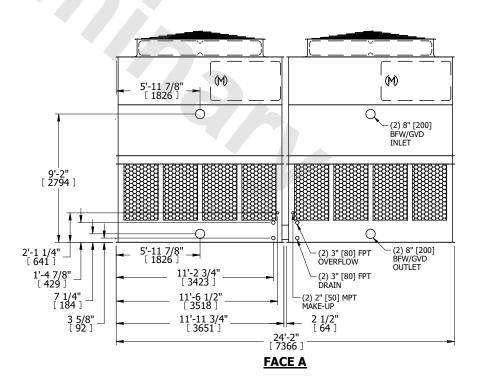
SHIPPING WEIGHT 15180 lbs+ [6890] kg+ OPERATING WEIGHT 27600 lbs+ [12520] kg+ HEAVIEST SECTION WEIGHT 5050 lbs+ [2295] kg+ NO. OF SHIPPING SECTIONS 4 DRAWN BY: KDS
