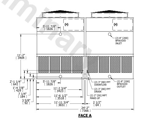
SHIPPING WEIGHT 17540 lbs+ [7960] kg+ OPERATING WEIGHT 29960 lbs+ [13590] kg+ HEAVIEST SECTION WEIGHT 6230 lbs+ [2830] kg+ NO. OF SHIPPING SECTIONS 4 DRAWN BY: KDS
