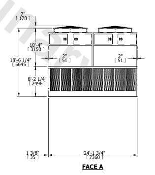
DRAWN BY: JLG NO. OF SHIPPING SECTIONS **SHIPPING** OPERATING HEAVIEST SECTION 6480 lbs+ [2940] kg+ 37500 lbs+ [17010] kg+ 61820 lbs+ [28045] kg+ WEIGHT WEIGHT WEIGHT
