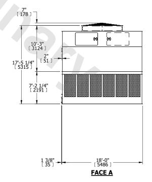
SHIPPING WEIGHT 21880 lbs+ [9925] kg+ OPERATING WEIGHT 37080 lbs+ [16820] kg+ HEAVIEST SECTION WEIGHT 7030 lbs+ [3190] kg+ NO. OF SHIPPING SECTIONS 4 DRAWN BY: KDS
