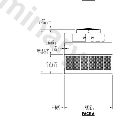
SHIPPING WEIGHT 20720 lbs+ [9400] kg+ OPERATING WEIGHT 35920 lbs+ [16295] kg+ HEAVIEST SECTION WEIGHT 6450 lbs+ [2930] kg+ NO. OF SHIPPING SECTIONS 4 DRAWN BY: JLG
