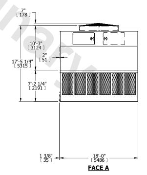
SHIPPING WEIGHT 22780 lbs+ [10335] kg+ OPERATING WEIGHT 37980 lbs+ [17230] kg+ HEAVIEST SECTION WEIGHT 7480 lbs+ [3395] kg+ NO. OF SHIPPING SECTIONS 4 DRAWN BY: KDS
