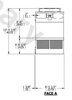
SHIPPING WEIGHT 8500 lbs+ [3860] kg+ OPERATING WEIGHT 13340 lbs+ [6055] kg+ HEAVIEST SECTION WEIGHT 2910 lbs+ [1320] kg+ NO. OF SHIPPING SECTIONS 4 DRAWN BY: JLG
