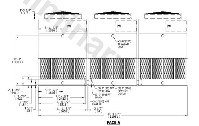
SHIPPING WEIGHT 23790 lbs+ [10795] kg+ OPERATING WEIGHT 38840 lbs+ [17620] kg+ HEAVIEST SECTION WEIGHT 5220 lbs+ [2370] kg+ NO. OF SHIPPING SECTIONS 6 DRAWN BY: JLG
