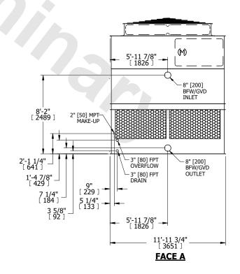
DRAWN BY: KDS NO. OF SHIPPING SECTIONS **SHIPPING** OPERATING HEAVIEST SECTION 7330 lbs+ [3325] kg+ 4930 lbs+ [2240] kg+ 13540 lbs+ [6145] kg+ WEIGHT WEIGHT WEIGHT
