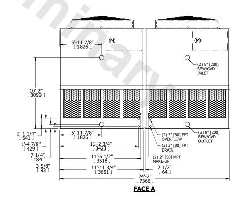
SHIPPING WEIGHT 15880 lbs+ [7205] kg+ OPERATING WEIGHT 28300 lbs+ [12840] kg+ HEAVIEST SECTION WEIGHT 5400 lbs+ [2450] kg+ NO. OF SHIPPING SECTIONS 4 DRAWN BY: KDS
