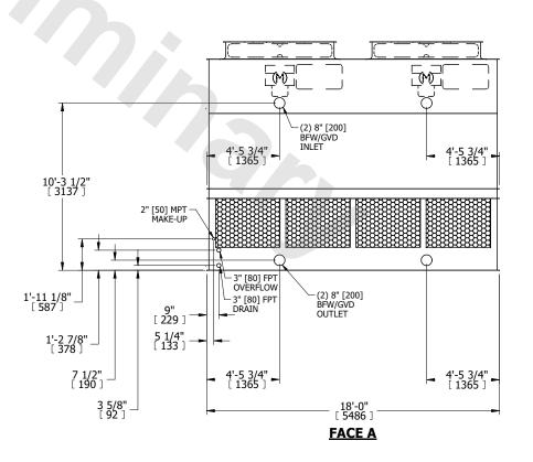
SHIPPING WEIGHT 9360 lbs+ [4250] kg+ OPERATING WEIGHT 15250 lbs+ [6920] kg+ HEAVIEST SECTION WEIGHT 6540 lbs+ [2970] kg+ NO. OF SHIPPING SECTIONS 2 DRAWN BY: JLG
