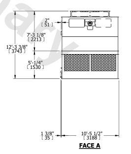
SHIPPING WEIGHT 9560 lbs+ [4340] kg+ OPERATING WEIGHT 16160 lbs+ [7335] kg+ HEAVIEST SECTION WEIGHT 3060 lbs+ [1390] kg+ NO. OF SHIPPING SECTIONS 4 DRAWN BY: JLG
