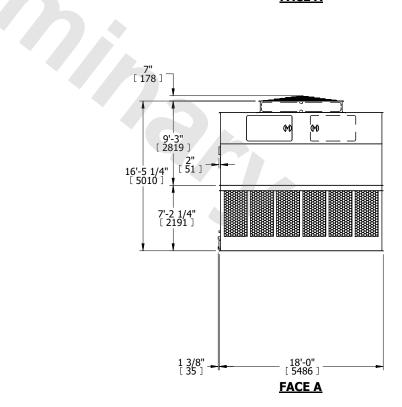
SHIPPING WEIGHT 20620 lbs+ [9355] kg+ OPERATING WEIGHT 35820 lbs+ [16250] kg+ HEAVIEST SECTION WEIGHT 6400 lbs+ [2905] kg+ NO. OF SHIPPING SECTIONS 4 DRAWN BY: JLG
