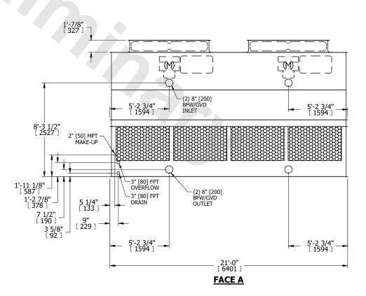
DRAWN BY: JLG SHIPPING NO. OF SHIPPING SECTIONS OPERATING HEAVIEST SECTION 9460 lbs+ [4295] kg+ 16400 lbs+ [7440] kg+ 6270 lbs+ [2845] kg+ WEIGHT WEIGHT WEIGHT
