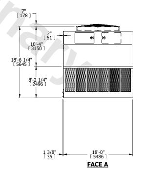
SHIPPING WEIGHT 26160 lbs+ [11870] kg+ OPERATING WEIGHT 44700 lbs+ [20280] kg+ HEAVIEST SECTION WEIGHT 8700 lbs+ [3950] kg+ NO. OF SHIPPING SECTIONS 4 DRAWN BY: KDS
