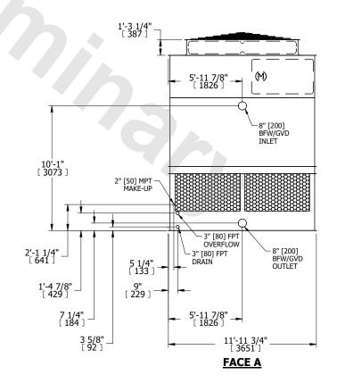
SHIPPING WEIGHT 7520 lbs+ [3415] kg+ OPERATING WEIGHT 12480 lbs+ [5665] kg+ HEAVIEST SECTION WEIGHT 5100 lbs+ [2315] kg+ NO. OF SHIPPING SECTIONS 2 DRAWN BY: JLG
