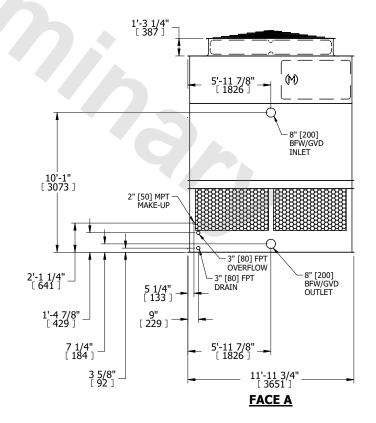
SHIPPING WEIGHT 7590 lbs+ [3445] kg+ OPERATING WEIGHT 12550 lbs+ [5695] kg+ HEAVIEST SECTION WEIGHT 5170 lbs+ [2350] kg+ NO. OF SHIPPING SECTIONS 2 DRAWN BY: JLG
