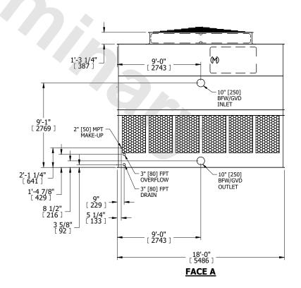
SHIPPING WEIGHT 11080 lbs+ [5030] kg+ OPERATING WEIGHT 20350 lbs+ [9235] kg+ HEAVIEST SECTION WEIGHT 7180 lbs+ [3260] kg+ NO. OF SHIPPING SECTIONS 2 DRAWN BY: KDS
