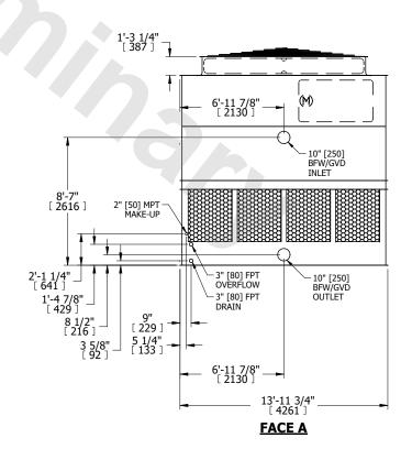
DRAWN BY: KDS NO. OF SHIPPING SECTIONS **SHIPPING** OPERATING HEAVIEST SECTION 8360 lbs+ [3795] kg+ 5490 lbs+ [2495] kg+ 15690 lbs+ [7120] kg+ WEIGHT WEIGHT WEIGHT
