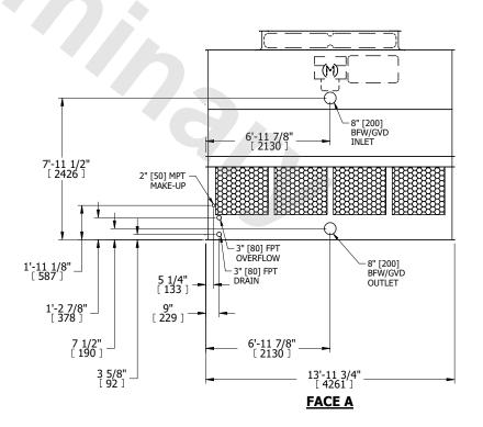
SHIPPING WEIGHT 5900 lbs+ [2680] kg+ OPERATING WEIGHT 10410 lbs+ [4725] kg+ HEAVIEST SECTION WEIGHT 3850 lbs+ [1750] kg+ NO. OF SHIPPING SECTIONS 2 DRAWN BY: JLG
