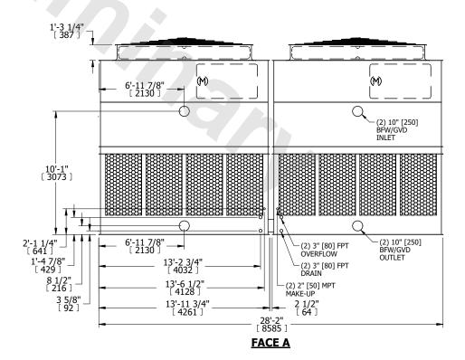
SHIPPING WEIGHT 16960 lbs+ [7695] kg+ OPERATING WEIGHT 31620 lbs+ [14345] kg+ HEAVIEST SECTION WEIGHT 5430 lbs+ [2465] kg+ NO. OF SHIPPING SECTIONS 4 DRAWN BY: KDS
