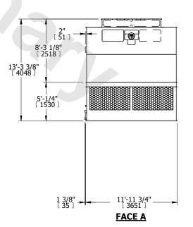
DRAWN BY: KDS NO. OF SHIPPING SECTIONS **SHIPPING** OPERATING HEAVIEST SECTION 11280 lbs+ [5120] kg+ 19000 lbs+ [8620] kg+ 3790 lbs+ [1720] kg+ WEIGHT WEIGHT WEIGHT
