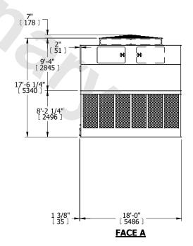
DRAWN BY: KDS NO. OF SHIPPING SECTIONS **SHIPPING** OPERATING HEAVIEST SECTION 23720 lbs+ [10760] kg+ 42260 lbs+ [19170] kg+ 7480 lbs+ [3395] kg+ WEIGHT WEIGHT WEIGHT
