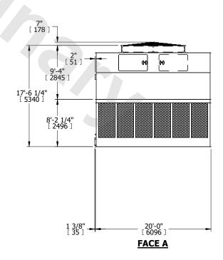
SHIPPING WEIGHT 26080 lbs+ [11830] kg+ OPERATING WEIGHT 46880 lbs+ [21265] kg+ HEAVIEST SECTION WEIGHT 8420 lbs+ [3820] kg+ NO. OF SHIPPING SECTIONS 4 DRAWN BY: BLL
