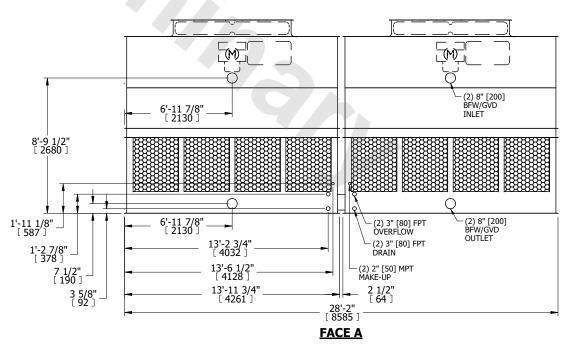
SHIPPING WEIGHT 11640 lbs+ [5280] kg+ OPERATING WEIGHT 20660 lbs+ [9375] kg+ HEAVIEST SECTION WEIGHT 3680 lbs+ [1670] kg+ NO. OF SHIPPING SECTIONS 4 DRAWN BY: JLG
