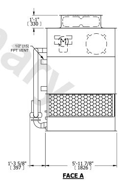
DRAWN BY: NO. OF SHIPPING SECTIONS **SHIPPING** OPERATING HEAVIEST SECTION 3160 lbs+ [1435] kg+ 4810 lbs+ [2185] kg+ 2650 lbs+ [1205] kg+ WEIGHT WEIGHT WEIGHT
