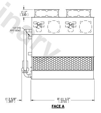
DRAWN BY: NO. OF SHIPPING SECTIONS **SHIPPING OPERATING** HEAVIEST SECTION 4600 lbs+ [2090] kg+ 3930 lbs+ [1785] kg+ 6990 lbs+ [3175] kg+ WEIGHT WEIGHT WEIGHT
