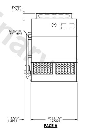
NO. OF SHIPPING SECTIONS **SHIPPING** OPERATING HEAVIEST SECTION 11690 lbs+ [5305] kg+ 10250 lbs+ [4650] kg+ 16930 lbs+ [7680] kg+ WEIGHT WEIGHT WEIGHT
