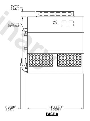
DRAWN BY: SLR NO. OF SHIPPING SECTIONS **SHIPPING OPERATING** HEAVIEST SECTION 11430 lbs+ [5185] kg+ 13230 lbs+ [6005] kg+ 19790 lbs+ [8980] kg+ WEIGHT WEIGHT WEIGHT
