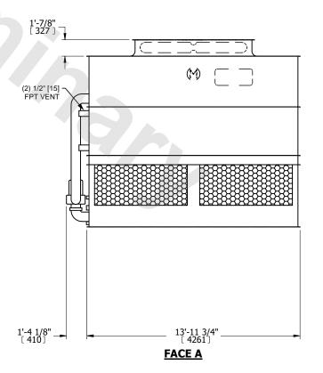
DRAWN BY: SLR NO. OF SHIPPING SECTIONS **SHIPPING** OPERATING HEAVIEST SECTION 13250 lbs+ [6015] kg+ 20220 lbs+ [9175] kg+ 11240 lbs+ [5100] kg+ WEIGHT WEIGHT WEIGHT
